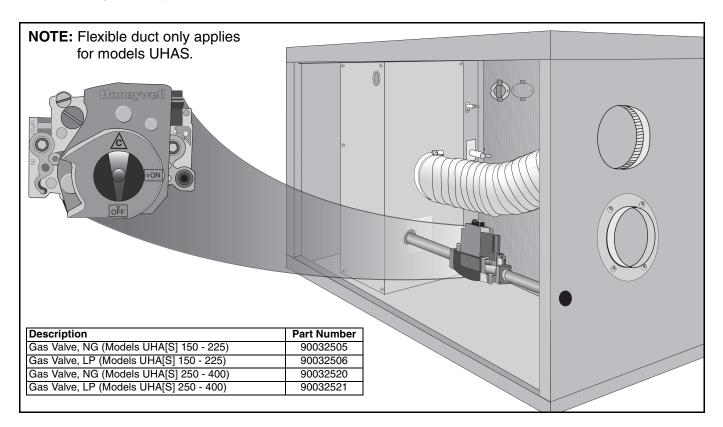
Follow steps in *Section 14.2* and *See Page 32, Section 14.2.1* to remove gas valve/manifold.
